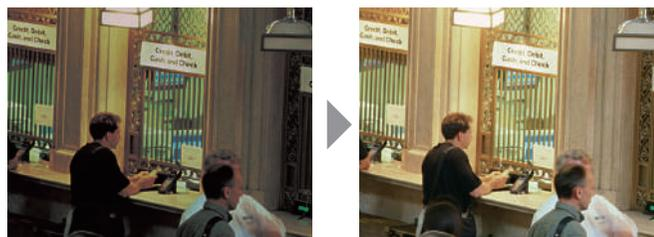
F/1.0 lens has two times light gathering power compared to F/1.4 making a 1 lux camera sensitivity into a 0.5 lux sensitivity.
